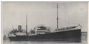
M.S. "BULYSSER" (Oil Tanker) Owners: Anglo-Saxon Petroleum Co. Shipbuilders: Hawthorn, Leslie and Co. Engine builders: Hawthorn, Leslie and Co. Speed: 10 1/2 knots. Deadweight capacity: 10,000 tons. Machinery: Sulphuric Hawthorn, Leslie. Workgear type four-cylinder double-acting engine. Output: 1,000 h.p.
